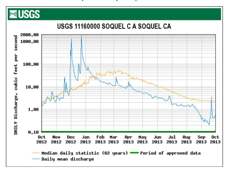
Figure 38. The March–May 2013 Discharge of Record for the USGS Gage on Soquel Creek at Soquel Village.
