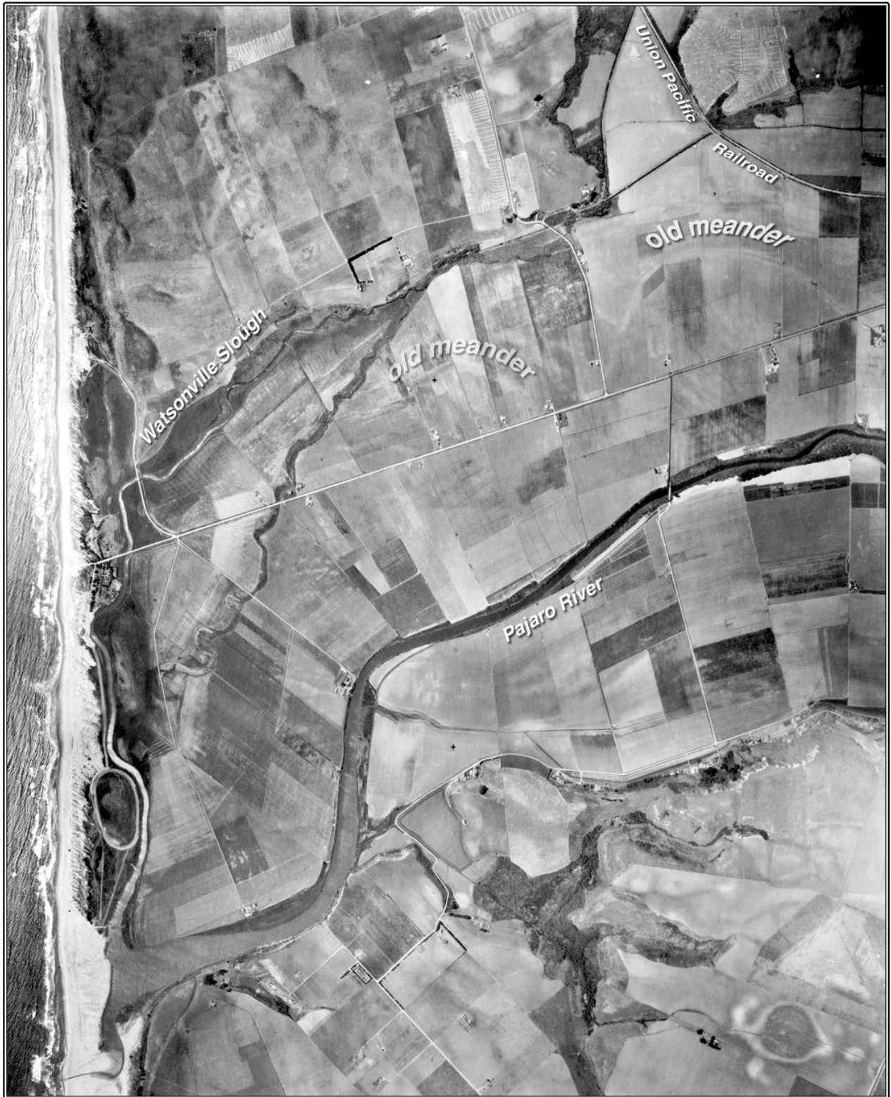
Figure 2-6: Aerial photograph of the lower reaches of Watsonville Slough and Pajaro River showing relic channel patterns and modifications to channel locations. Photo taken in 1931.
